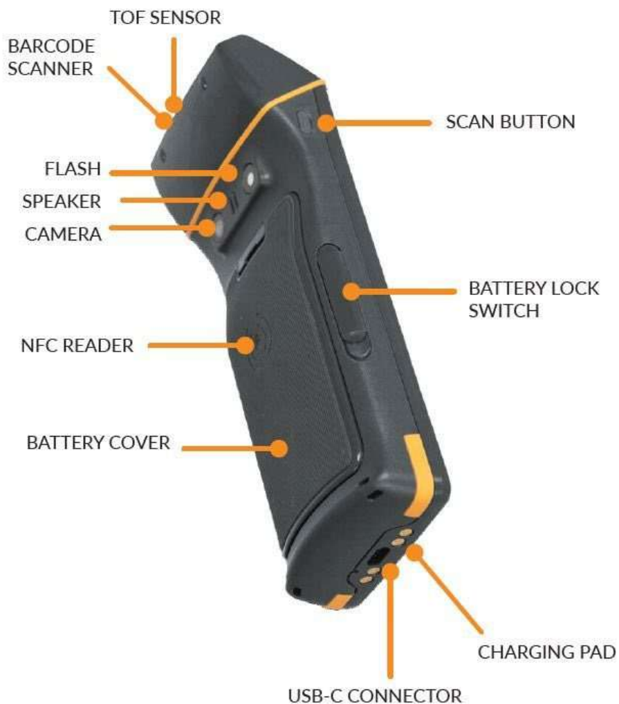
Picture 6 Features of Nordic ID HH83 (back side)
